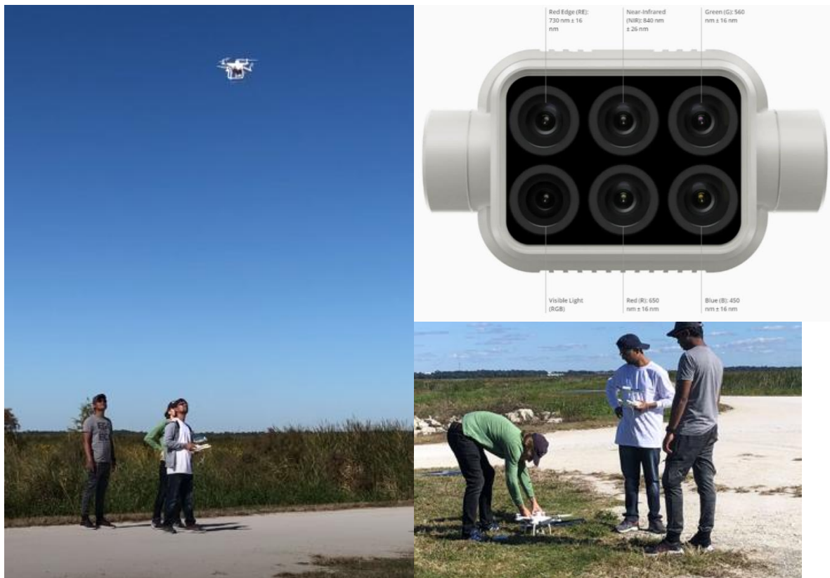
Figure 1. The DJI P4M drone operated by FAU students in the field (left, and right bottom), and the five multispectral cameras and 1 RGB camera onboard the DJI P4M drone (right top).
